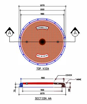
Specification : C250  $\varnothing$ 900 PSE-SMC Composite manhole cover
