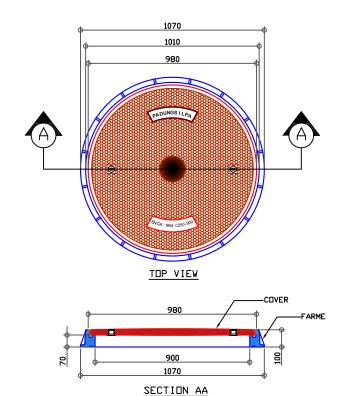
Specification: C250 Ø900 PSE-SMC Composite manhole cover
